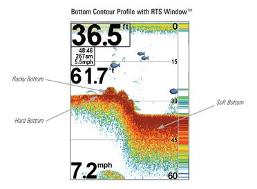
The sonar returns from the bottom, structure, and fish can be represented as either **WhiteLine**<sup>TM</sup> or **Structure ID**<sup>®</sup>. See *Sonar Menu Tab: Bottom View* for details on how to set the bottom view.
