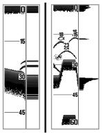
The Wide BTS Window™ indicates the sonar intensity through the use of a bar graph. The length of the plotted return indicates whether the return is weak or strong. The depth of the sonar return is indicated by the vertical placement of the return on the display depth scale The Wide RTS Window<sup>™</sup> does not use grayscale.
