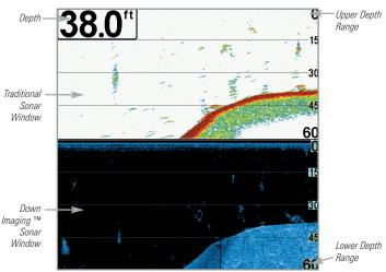
Down Imaging<sup>™</sup>/Sonar Combo View
