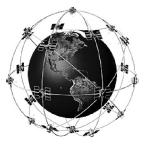
GPS uses a constellation of satellites that continually send radio signals to the earth. The GPS receiver on your boat receives signals from satellites that are visible to it. Based on time differences between each received signal, the GPS receiver determines its distance to each satellite. With distances known, the GPS receiver mathematically triangulates its own position. With once per second updates, the GPS receiver then calculates its velocity and bearing.
