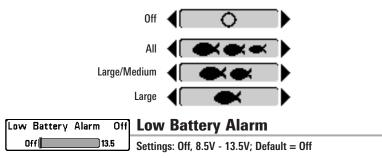
**Low Battery Alarm** sounds when the input battery voltage is equal to or less than the menu setting. The battery alarm will only sound for the battery that is connected to the Fishfinder. The Low Battery Alarm should be set to warn you when the battery voltage drops below the safety margin that you have determined.
