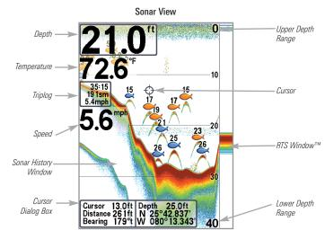
**NOTE:** If the Depth number is flashing, it means that the unit is having trouble locating the bottom. This usually happens if the water is too deep, the transducer is out of the water, the boat is moving too fast, or for any other reason that the unit can't accurately receive continuous data.
